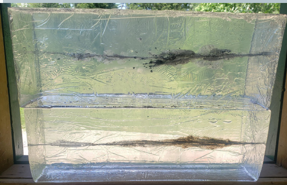
Comparing lead ammo fragmentation (top) and non-lead ammo fragmentation (bottom) using ballistic gels
